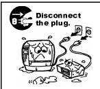
If foreign objects (metal fragments, water, liquids) enter the machines, first turn off the power switches and disconnect the power cord plugs from the outlet, and then contact your authorised TOSHIBA TEC representative for assistance. Continued use of the machine in that condition may cause **fire** or **electric shock**.
